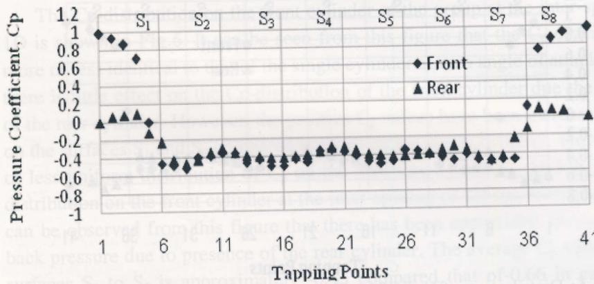
Figure 9: Distribution of  $C_p$  on front & rear cylinder at inter-spacing of 4D.
