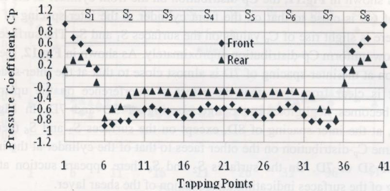
Figure 11: Distribution of  $C_p$  on front & rear cylinder at inter-spacing of 6D.
