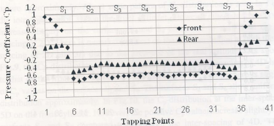
Figure 10: Distribution of  $C_p$  on front & rear cylinder at inter-spacing of 5D.
