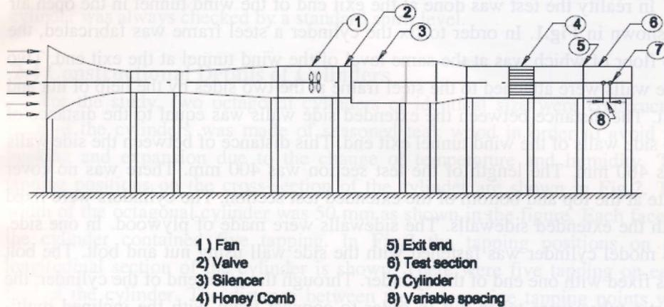
**Figure 1:** Schematic diagram of wind tunnel.
