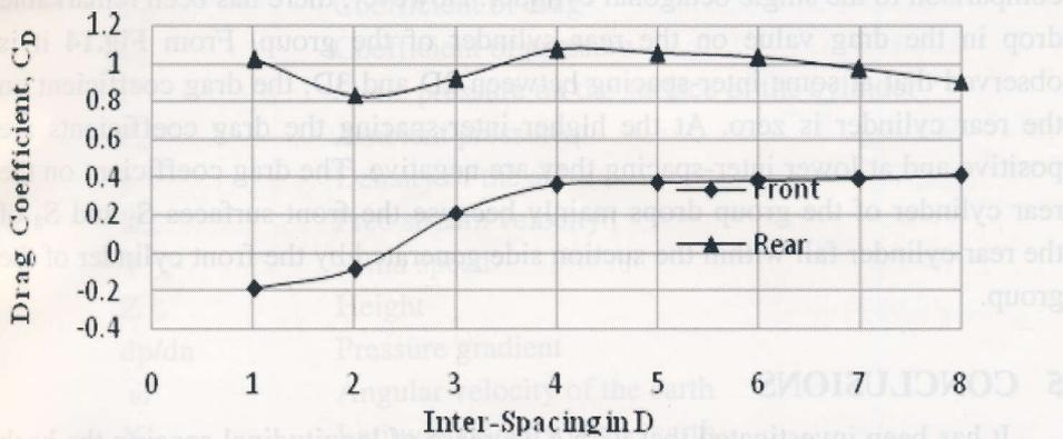
**Figure 14:** Variation of drag coefficient on front & rear cylinders at different inter-spacing.
