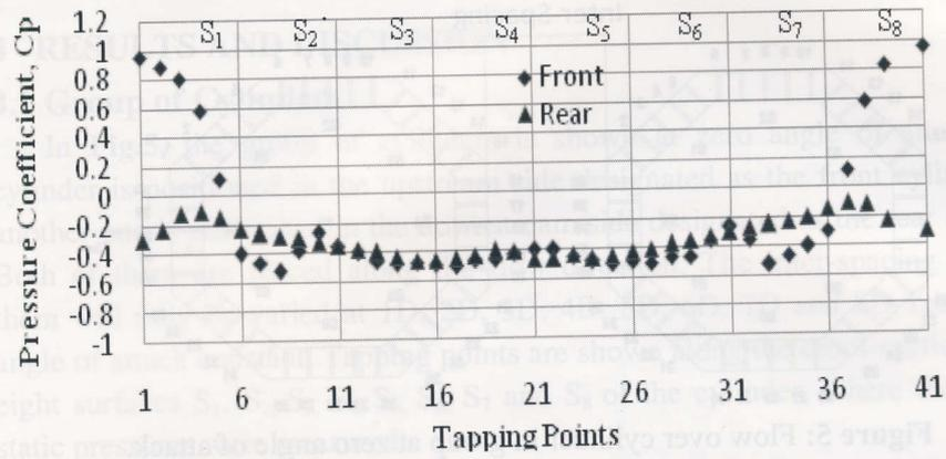
Figure 8: Distribution of  $C_p$  on front & rear cylinder at inter-spacing of 3D.
