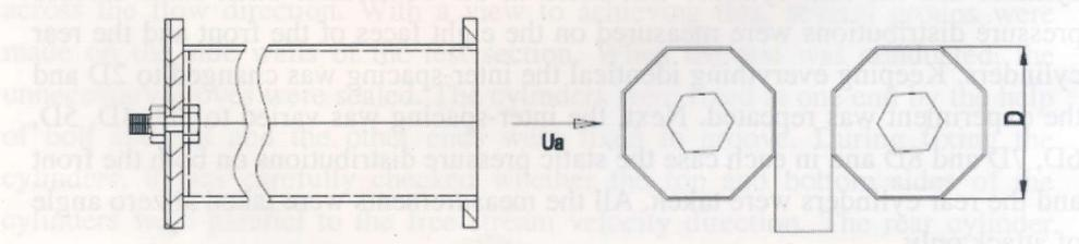
Figure 4: Tunnel test section showing position of group cylinders.
