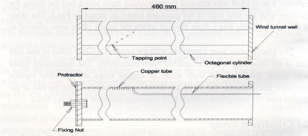
Figure 3: Tapping positions shown on longitudinal section of cylinder.
