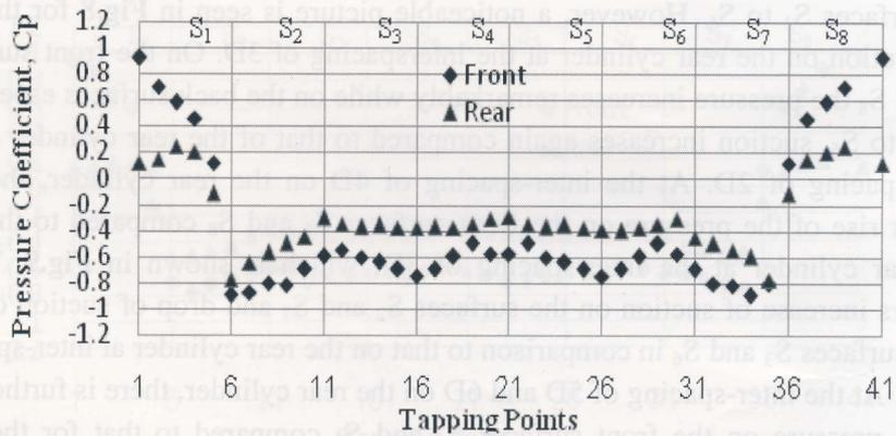
Figure 13: Distribution of  $C_p$  on front & rear cylinder at inter-spacing of 8D.
