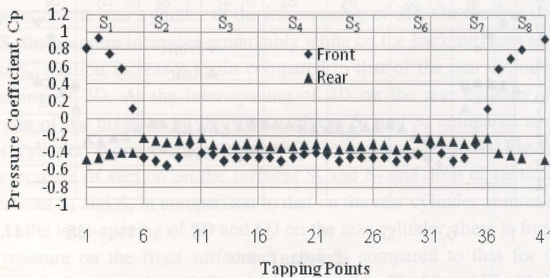
Figure 7: Distribution of  $C_p$  on front & rear cylinder at inter-spacing of 2D.
