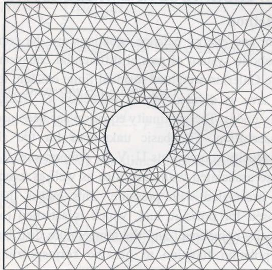
**Figure 2:** Mesh generation of the physical domain.
