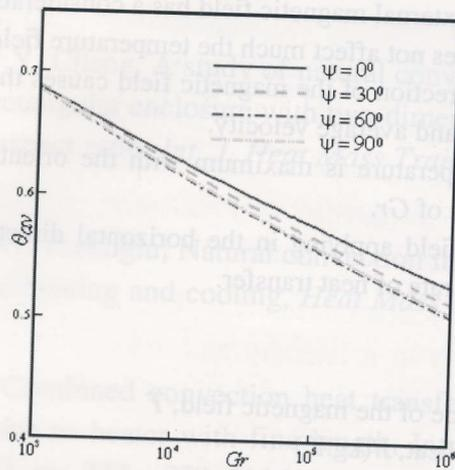
**Figure 6:** Average bulk temperature for different  $\psi$  along with  $Gr$ .
