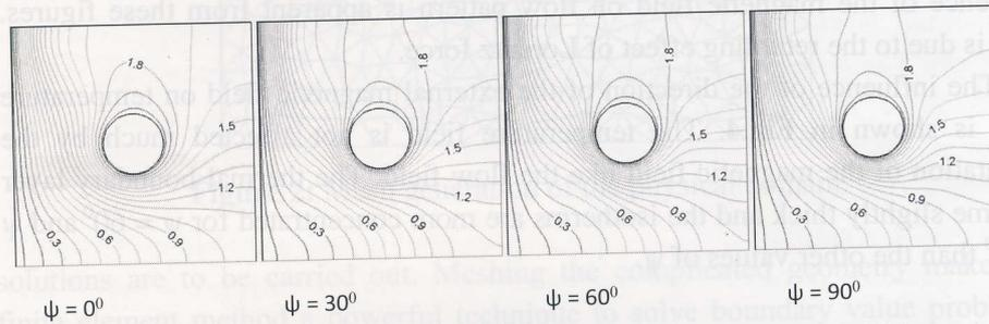
**Figure 4:** Isotherms for different angles of magnetic field made with horizontal direction.
