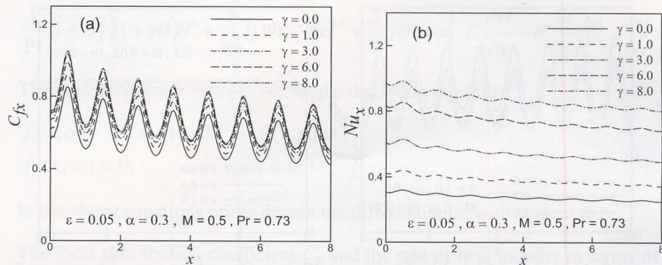
Figure 3: Variation of (a) skin friction coefficient  $C_{fx}$  and (b) rate of heat transfer  $Nu_x$  against  $x$  for different values of  $\gamma$  with  $\alpha = 0.3$ ,  $\epsilon = 0.05$ ,  $M = 0.5$  and  $Pr = 0.73$ .
