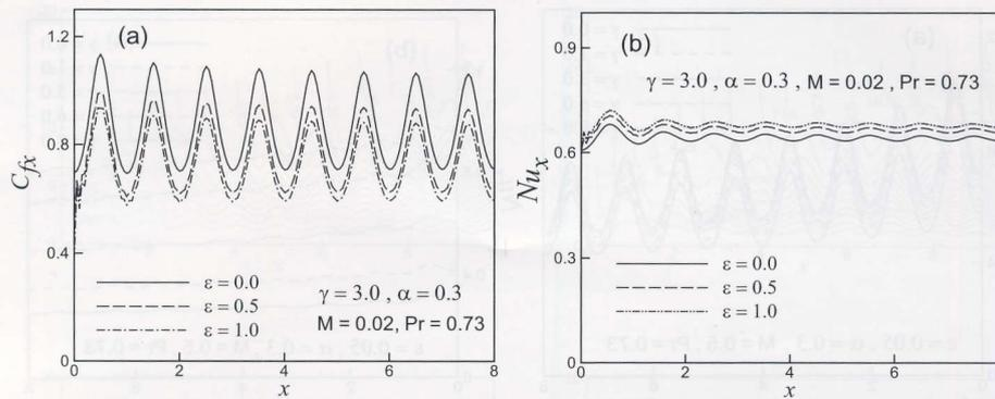
Figure 2: Variation of (a) skin friction coefficient  $C_{fx}$  and (b) rate of heat transfer  $Nu_x$  against  $x$  for different values of  $\epsilon$  with  $\alpha = 0.3$ ,  $M = 0.02$ ,  $\gamma = 3.0$  and  $Pr = 0.73$ .
