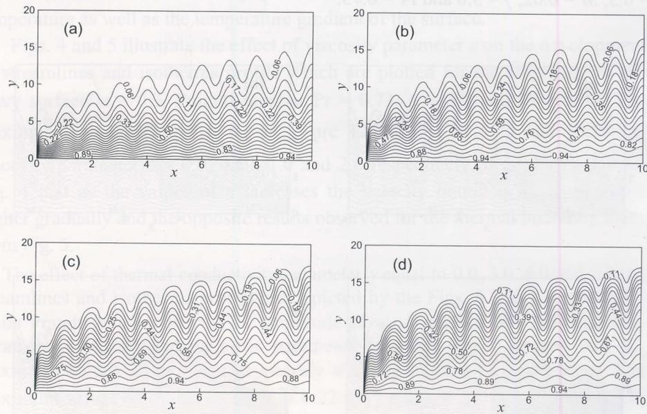
Figure 7: Isotherms for (a)  $\gamma = 0.0$  (b)  $\gamma = 1.0$  (c)  $\gamma = 3.0$  and (d)  $\gamma = 8.0$  while  $Pr = 0.73$ ,  $M = 0.5$ ,  $\varepsilon = 0.05$  and  $\alpha = 0.3$ .
