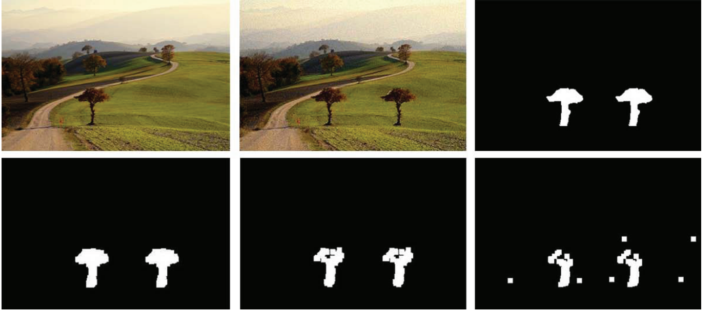
Fig. 6: Proposed method's performance for Gaussian noise. From top left to right: original image, forged image, ground truth; bottom left to right: proposed method result with SNR = 40, 30, 20 respectively.
