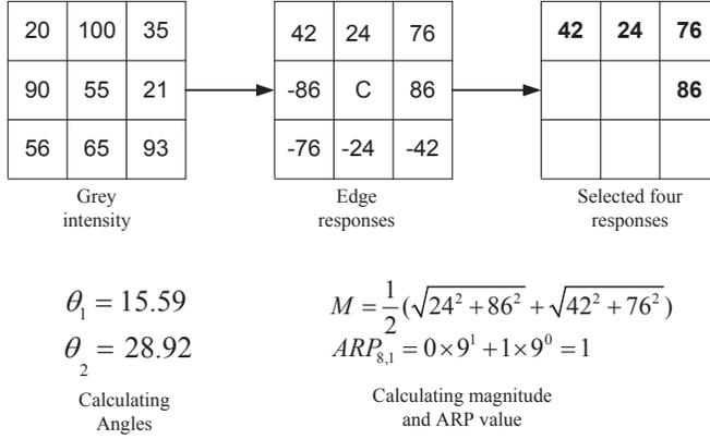
Fig. 3: Sample ARP value calculation.
