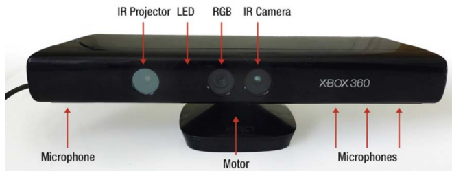
Fig. 1: Different Components of Microsoft Kinect [3], [4]
