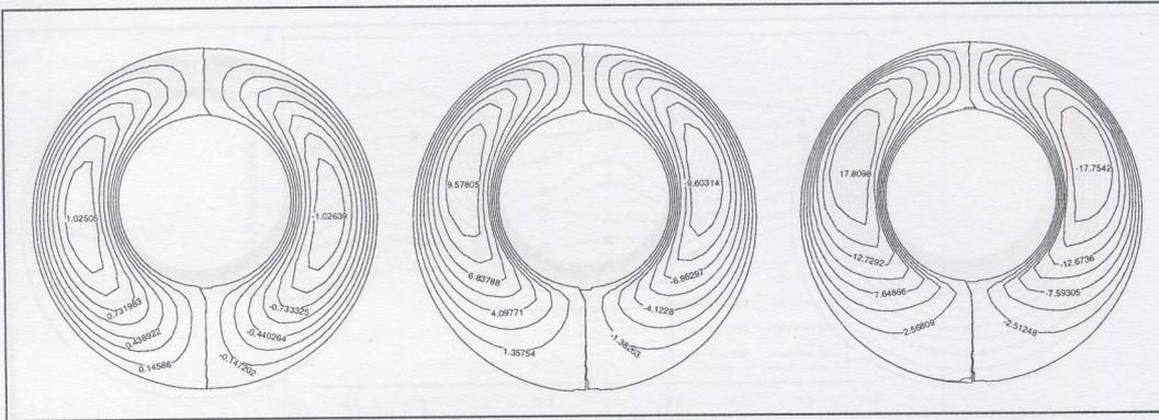
Fig. 1 Stream function contours for relative eccentricity of 0.2 and Rayleigh number of 10, 120 and 300 respectively
