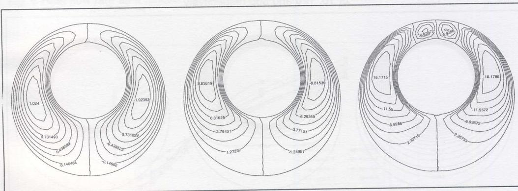
Fig. 3 Stream function contours for relative eccentricity of 0.5 and Rayleigh number of 10, 120 and 300 respectively
