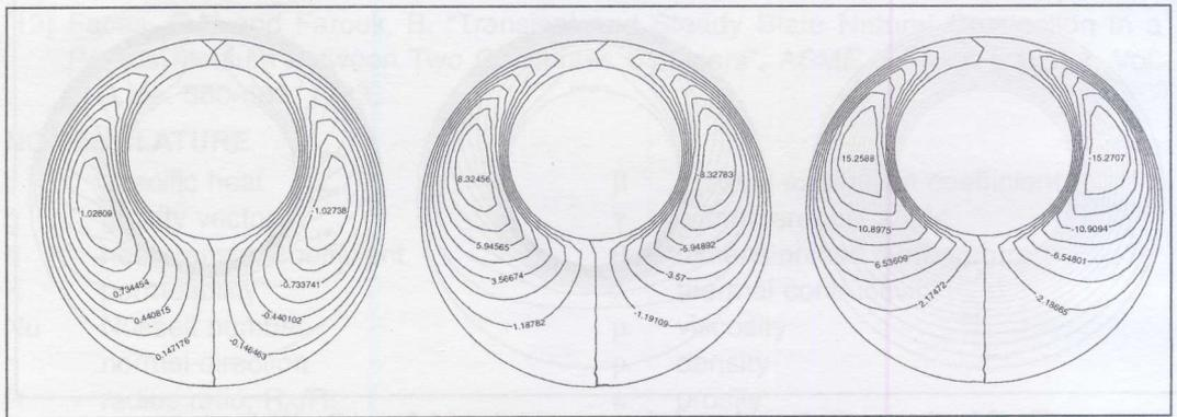
Fig. 5 Stream function contours for relative eccentricity of 0.7 and Rayleigh number of 10, 120 and 300 respectively
