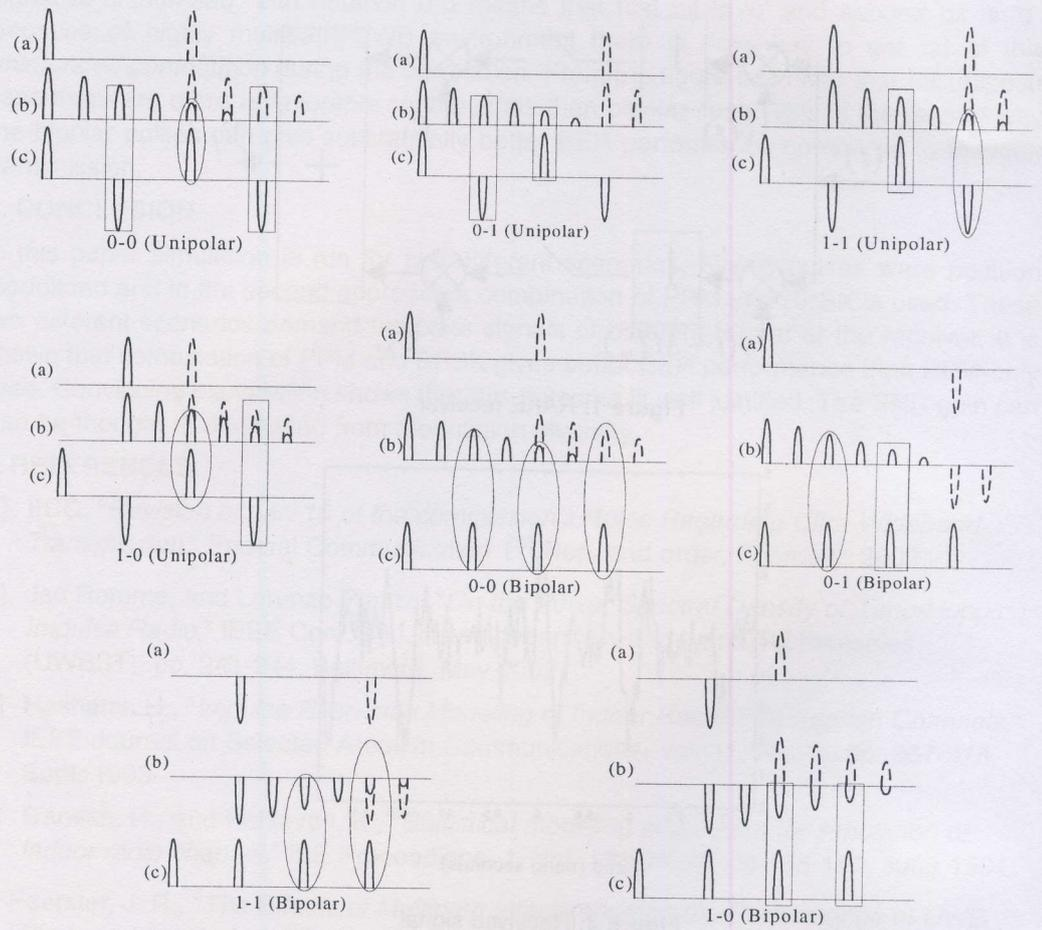
**Figure 4:** Schematic scenario at the first finger of the RAKE receiver
