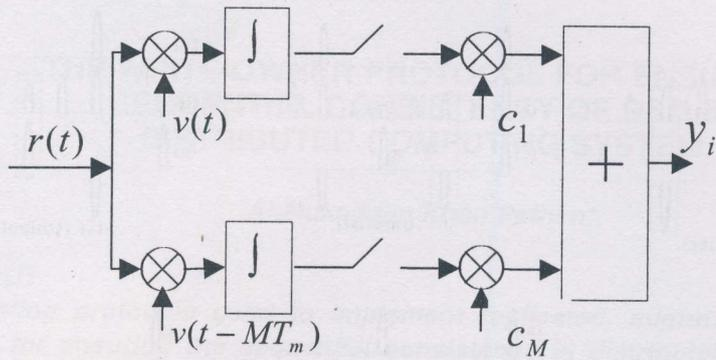
Figure 1: RAKE receiver
