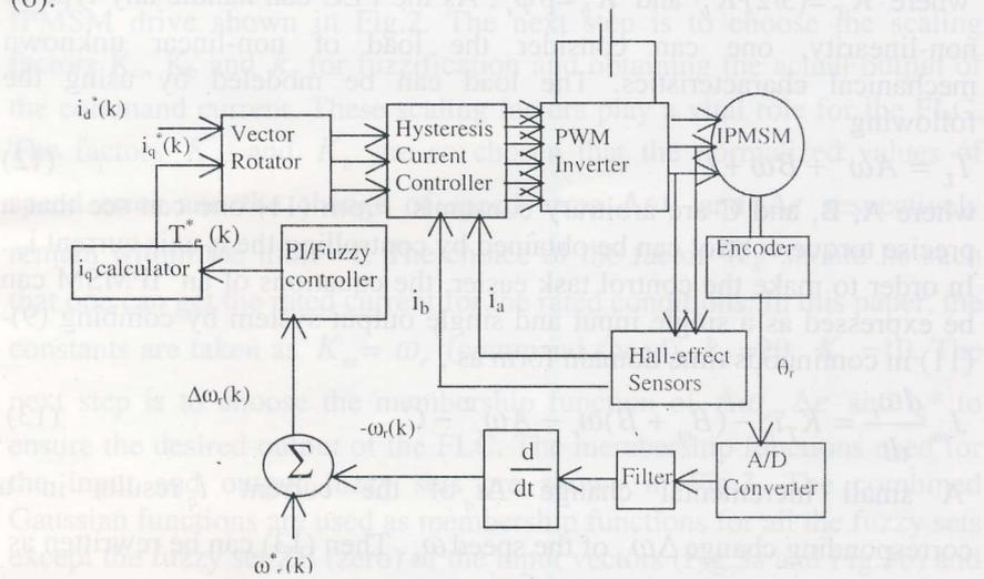
Fig.2 Block diagram for the proposed controller based IPMSM Drive.
