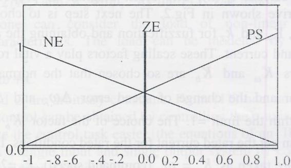
Fig.3 (c) Membership function for quadrature-axis current,  $i_q$
