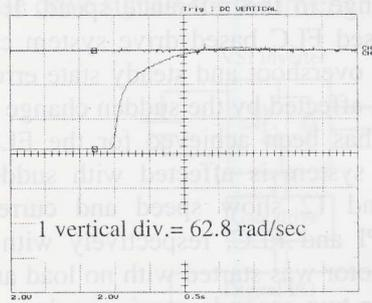
Fig. 7 (a) Experimental speed response at a load of 2 N-m with PI/MTPA
