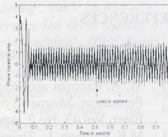
Fig. 12(b) Current responses at sudden change of load with fuzzy controller/MTPA
