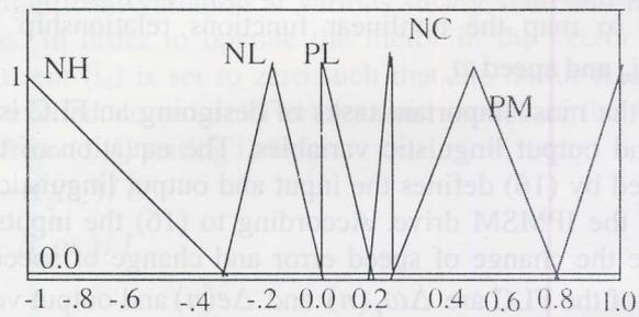
Fig. 3(b) Membership function for change of speed error  $\Delta e$  (n)
