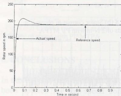
Fig. 5(a) Speed responses at a load of 2 N-m with PI controller/ MTPA
